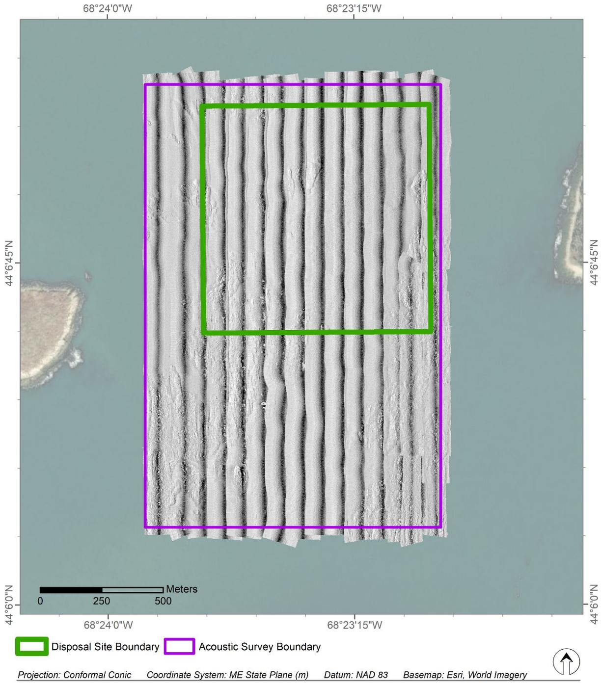
**Figure 3-10.** Side-scan sonar data at Frenchboro Disposal Site, 2022
