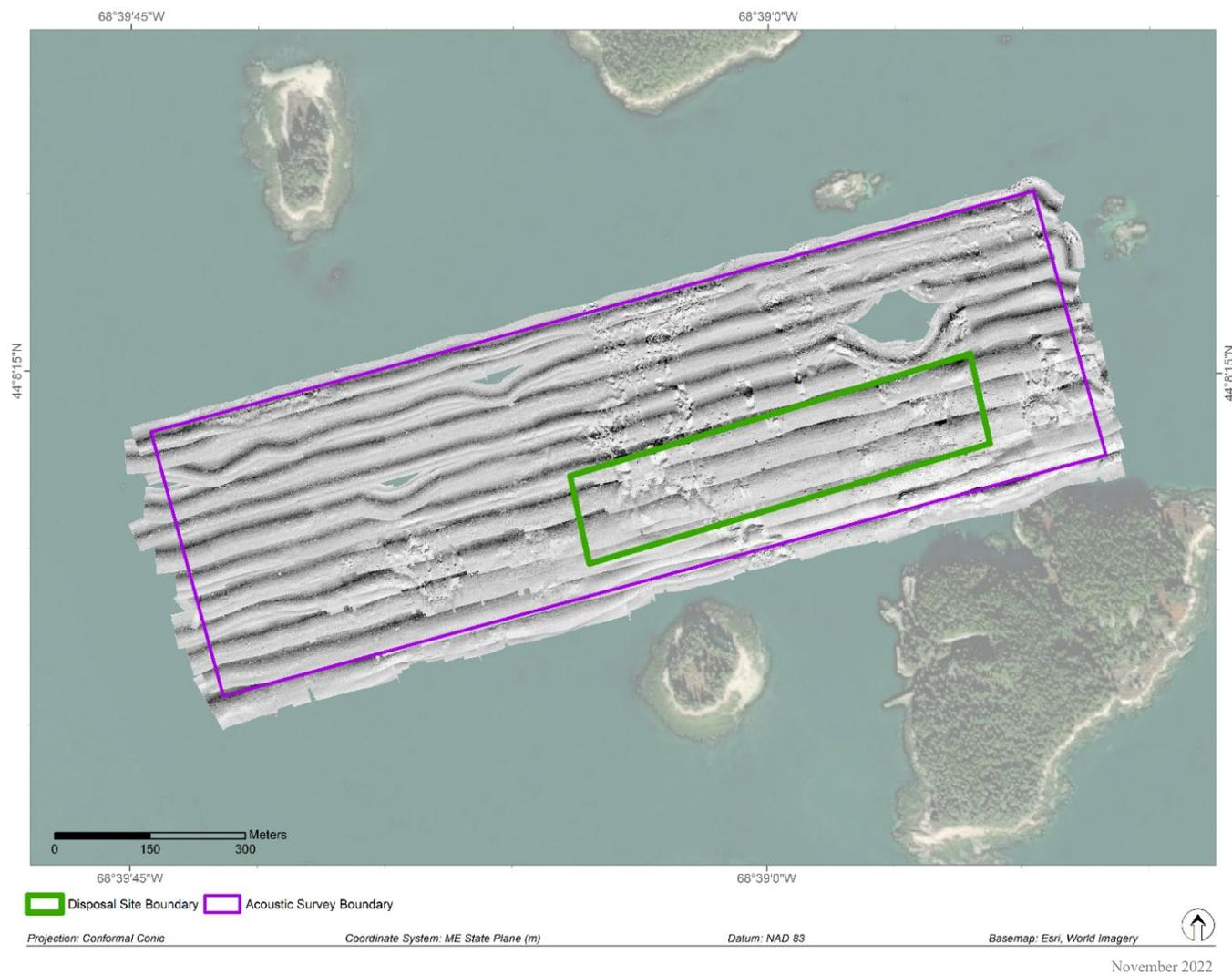
**Figure 3-4.** Side scan sonar data at SHDS, 2022
